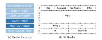
Figure 7: Segment routing header design.
